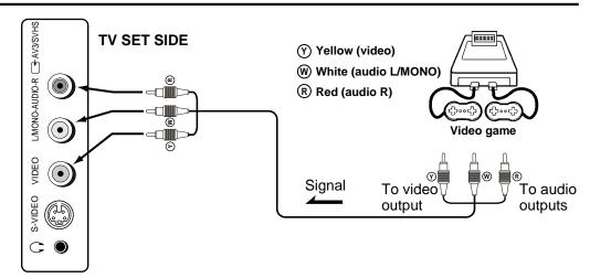
The figure below shows how to connect the SVHS input to video equipment.
